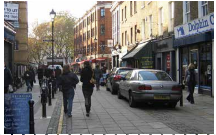
Shared Streets: Curbless streets, often with pavers designating user zones, that prioritize pedestrians and add to the public park space.
